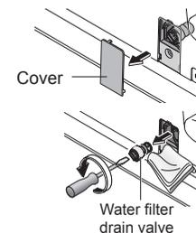
(4) After draining the water, install the water filter drain valve and cover. Insert the water filter drain valve and use a flat-head screwdriver to tighten it securely.
