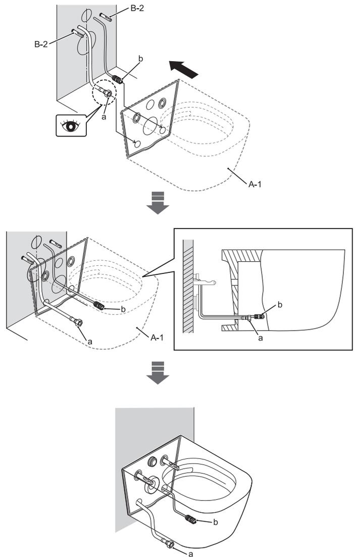
**Note:** When placing the toilet bowl, be careful not to pinch the water supply hose and electric wiring.
