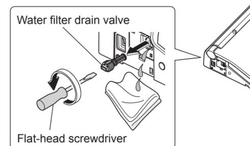
**5** When water draining is completed, reinstall the water filter drain valve.
