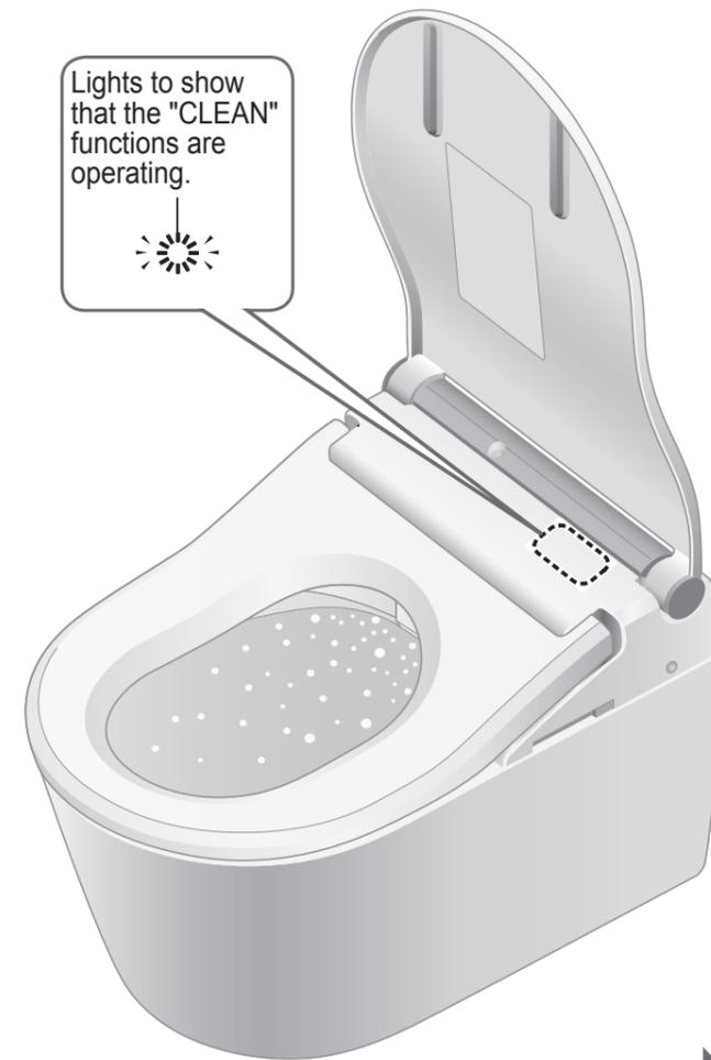
The self-cleaning functions operate automatically.
