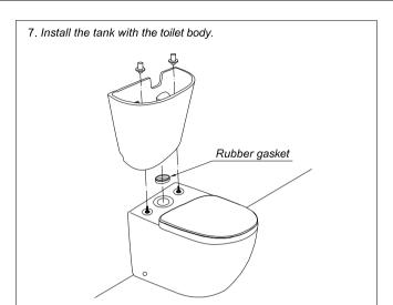
Note: Have to place the rubber gasket right into center of outlet hole. Otherwise may be water leakage.
